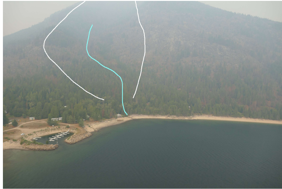
Photo 1: View looking northwest up the Tye Creek draw (creek in blue, watershed boundary in white). The Cultus Creek valley is visible at the left of the image. The boat basin and most of the recreational properties are on the Cultus Creek fluvial fan.
